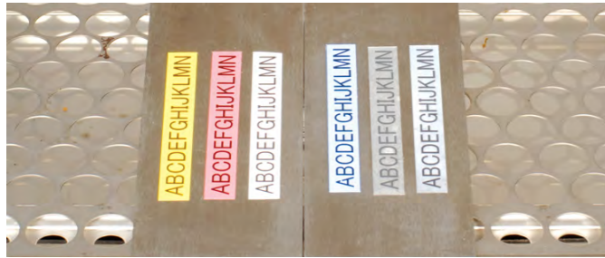
Temperature resistant: laminated labels were subjected to temperatures ranging from -80C to +150C for 240 hours, and the text was found to be unaffected.
